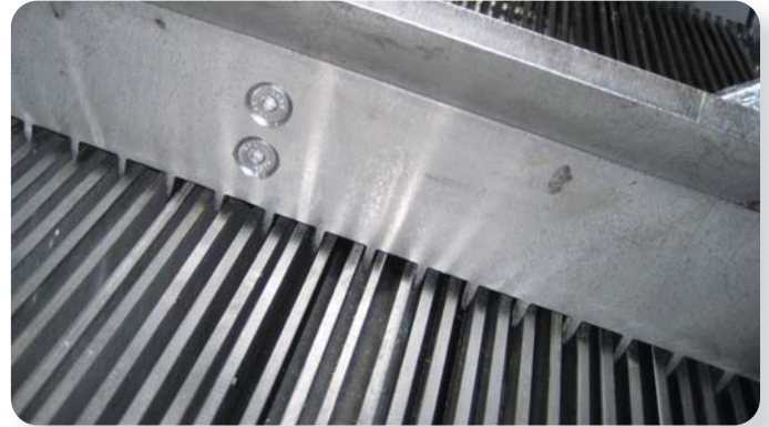
Alternate bar cleaning feature.
