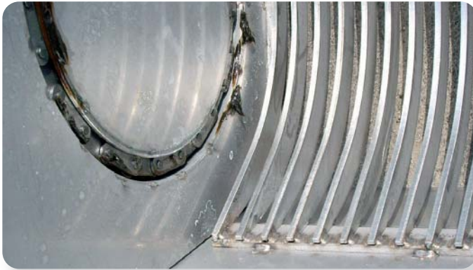
Chain and chain guide enclosure.
