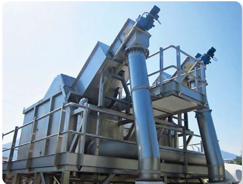
Three FD-MBR1400 3 MGD Per Screen - Trento Italy
