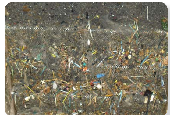
Screening mat enhances capture of fine solids.
